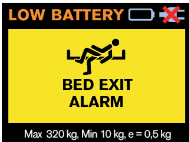
Fig. Visual signalisation of the Bed Exit Alarm on the display (yellow field and black symbols)
