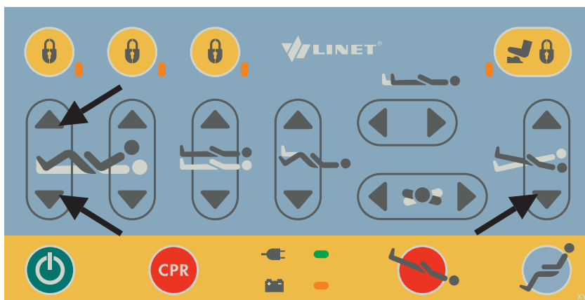
Fig. Deactivation of the accumulator (Attendant Control Panel)
