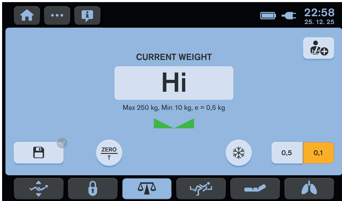
Fig. First level of the bed overload (displayed Hi)
