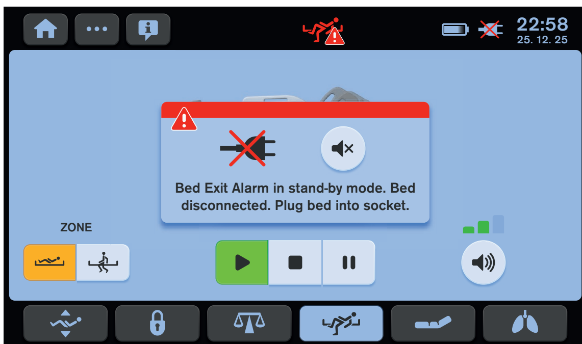
Fig. Bed Exit Alarm Monitoring is deactivated because of the bed disconnected from the mains power
