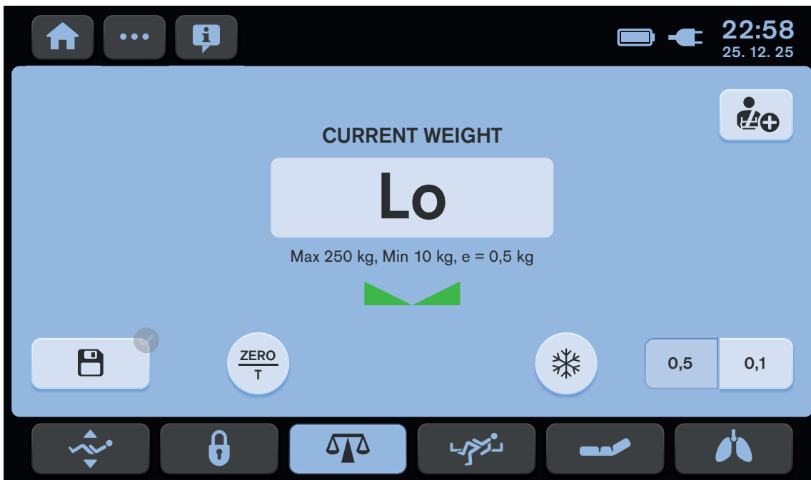
Fig. Underloaded bed (displayed Lo)
