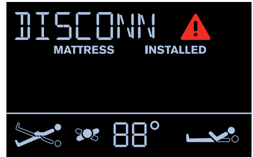
Fig. DISCONNECTED AIR PIPES
