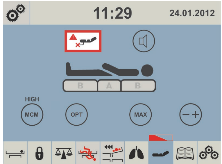
Fig. Alert – Disconnected Air Pipes
