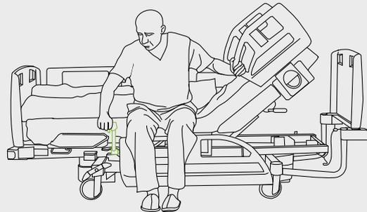
*The patient can slide out the Mobi-Lift® handle using one hand.*
